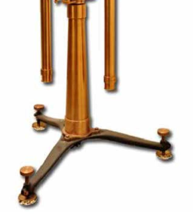
A new version of the torsion balance, having one weight hanging down from the end of the rod, was called horizontal variometer by Eötvös, because it made it possible to measure the horizontal gradient of g in addition to the direction and difference of the two main curvatures.
